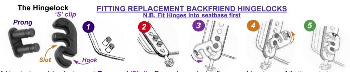
A hingelock consists of a two part **Prong** and 'S' clip. Remember no tools - fingers and hands are all that's needed. Hinges (see over) MUST be inserted correctly into seatbase BEFORE fitting hingelocks (for clarity seatbase not shown in images).
